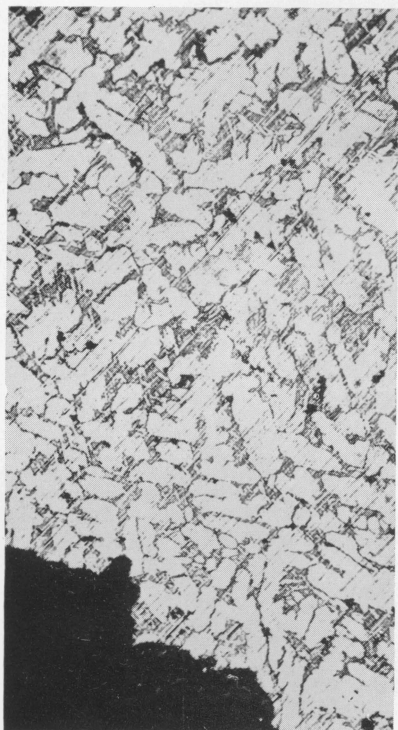
B. —Etched section of anvil. \times 80 .
