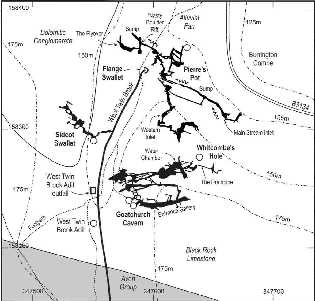
**Figure 8.** Simplified survey of Sidcot Swallet, Goatchurch Cavern and Pierre's Pot. Adapted from surveys published by UBSS and Mendip Caving Group.
