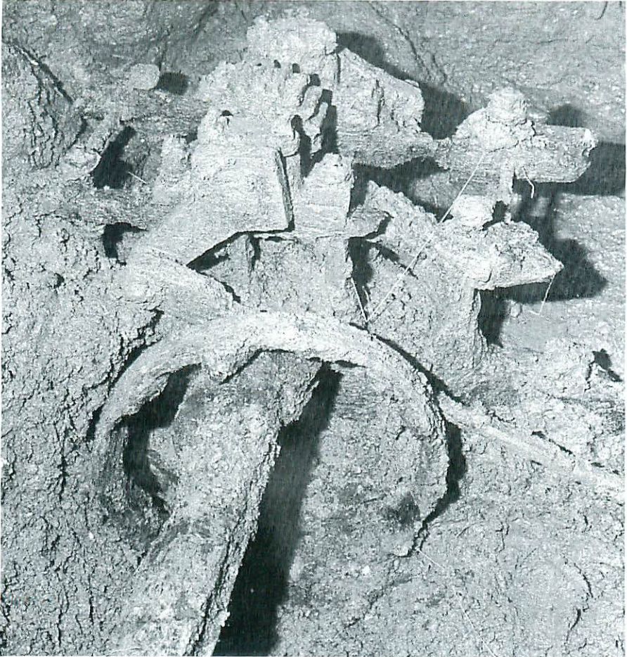
FIG. 13—THE AXLE AND GEARBOX PARTLY CLEARED OF MUD TAILINGS Phot.: N. R. Barrington
